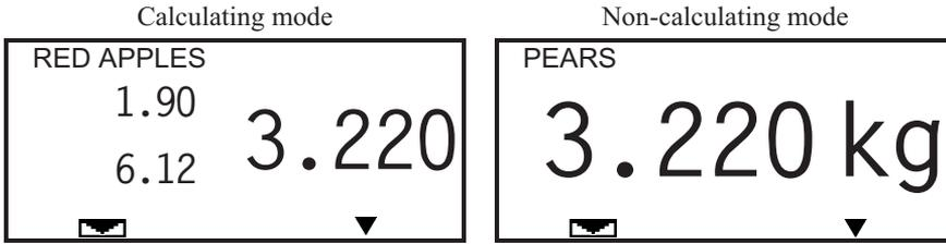
After weighing the commodity, understood as the stabilization of the positive result, and removing the load from the platter the scale will automatically reset the unit price and delete the product name from the display if they were previously inputted.
