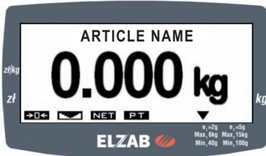
Selection of the display mode is automatic and depends on whether the unit price will be sent to the scale. After turning on the scale, the non-calculating mode is enabled (showing only the weight), after the first transfer of the unit price the mode switches to a calculating mode which remains active until powering off the scale. If only the article weight is displayed the scale transmits zero as a unit price and amount.
